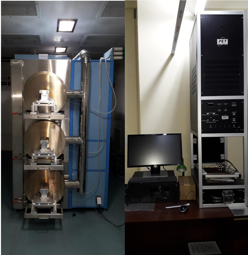
Oxidation-Diffusion Furnace (left) and Lifetime Measurement Unit (right) at the DST-IIEST Solar PV Hub
