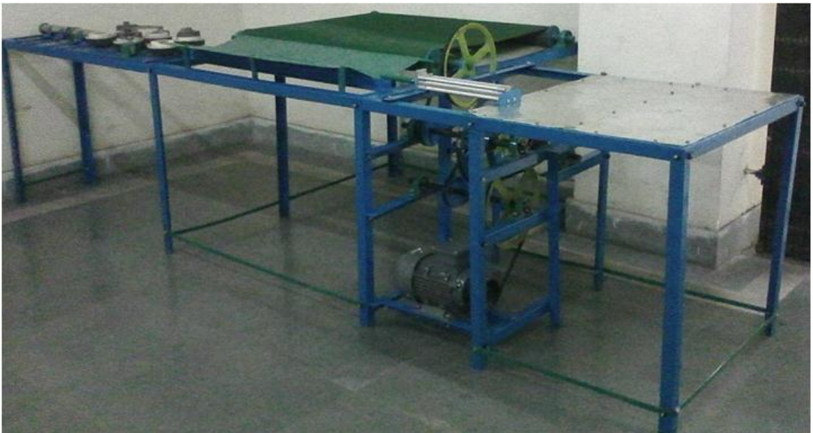
Semi-Automatic Jute Fibre Extraction Machine, development in progress, at the School of Mechatronics and Robotics
