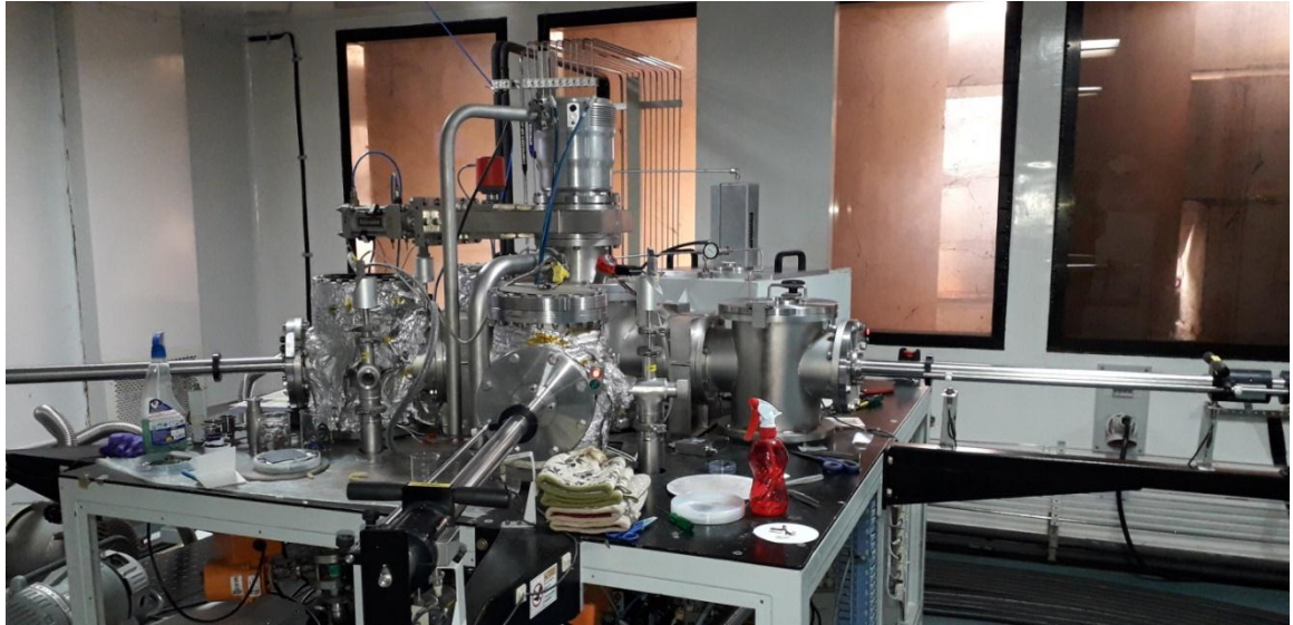
Plasma Enhanced Chemical Vapor Deposition (PECVD) Cluster Tool at DST-IIEST Solar PV-Hub
