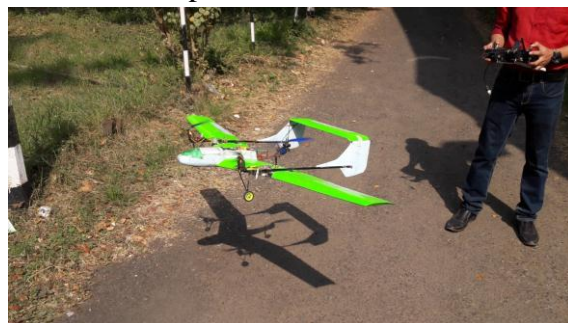
The VTOL aircraft, designed and developed as an experimental set-up for students at the Department of Aerospace and Applied Mechanics
